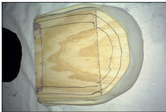
Marks on plywood base. The edge of the seat cover will have to be aligned between these marks.
