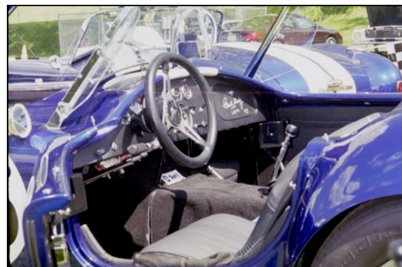
Cockpit of SP447 with reversed shifter, hand control under the leather wrapped steering wheel, and Carroll Shelby's signature on the glove box door.
