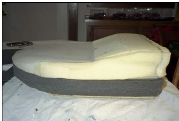
Seat with original foam, new foam, and plywood base.
