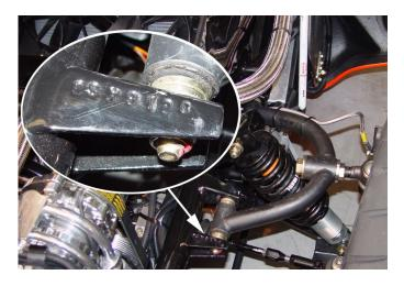
The CSX9000 chassis number is stamped on the rearmost frame mount for the right hand side upper front A-arm.
