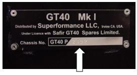
The GT40 **chassis number** plate shown above shows the chassis number as GT40-P-2192. The chassis number plate is typically attached to right hand side or left hand side of the firewall inside the engine compartment.
