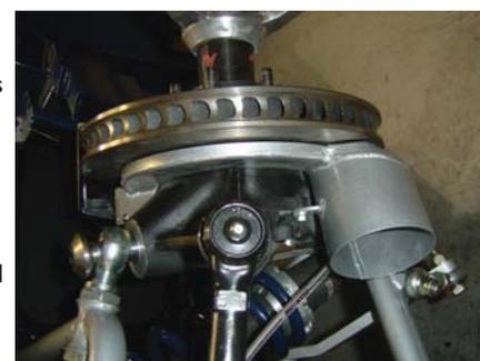
GT 40 Brake Ducts (Front and rear ) is \$600.00 including the flexible tubing. Note, the brake ducts clear the parking brake unit at the back of the car.
