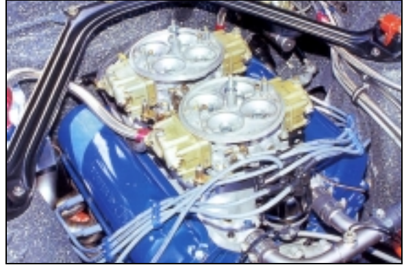
Figure 1: No end to excess. 1969 Trans-Am Boss 302 sporting 2 (!) 1050 cfm Holley Dominators.
