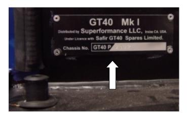
The chassis number plate is typically pop riveted by the dealer to right hand side or left hand side of the firewall inside the engine compartment. The chassis number plate above shows the chassis number as GT40 P/2192.
