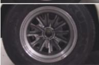
Superformance 17" Wheels (same as option offered on Superformance Mk III but drilled for 6 drive pins)
