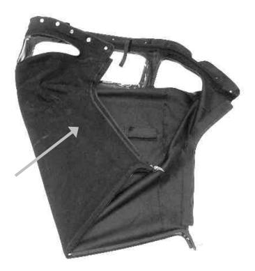
2. Fold the left half over as shown. Fold from between windows to center of front edge.
