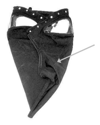
3. Fold the other side over as for Step 2. Keep rails as close as possible together. Be sure to turn the rails so that fabric at the junction of the rails is not under undue tension.
