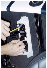
bracket. Only two mounting screws are required, but I elected to use 4 (more is better?). There were three pairs of holes. I elected to use the middle and lower pair. The upper pair is too high and would require drilling into the upper frame crossmember. I aligned the
