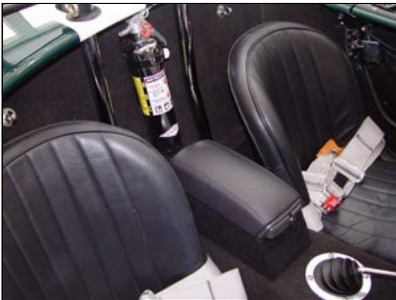
During an extended road-trip in upstate New York, Tony Revetti (SP 1085) realized there was something he needed in his Mk III. He built a custom fit, high quality center console incorporating key features for driver and passenger, as well as providing additional storage for the odds and ends that tended to litter our cars during longer road-trips.
