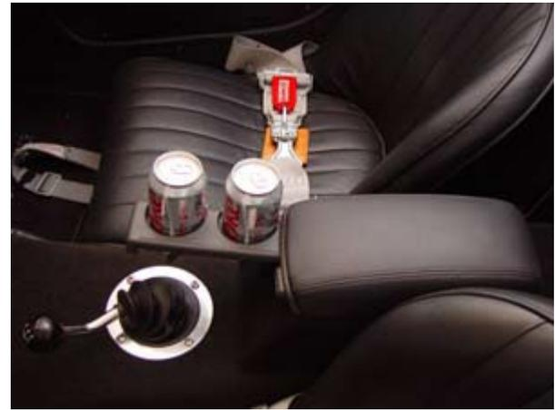
The left tab raises the lid. The right tab slides out to provide a two position cup holder.
