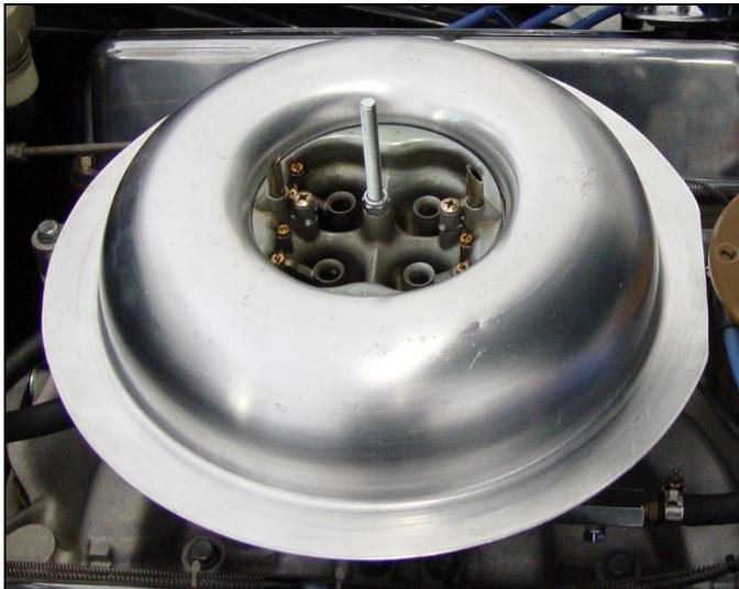
The domed top is contoured to match the base as can be seen from the domed shape and deeply recessed hold down nut.
