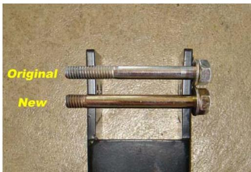
New 8mm, Class 10.9 bolts are available at Advanced Automotive Technologies Corporation 262-673-4077 <http://superformance.org/mountupgrade> or you can use 5/16" Grade 8 bolts from suppliers such as [www.aircraftspruce.com](http://www.aircraftspruce.com) part number AN5-27A
